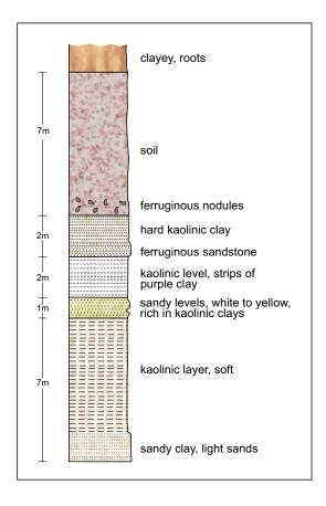
Figure 7 - Exploration Pits Composite Profile
