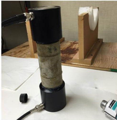
Figure 29. Transducers used to transmit and receive the compressional waves (P-waves) and the shear waves (S-waves) through the samples.
