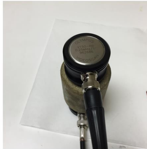
Figure 29. Transducers used to transmit and receive the compressional waves (P-waves) and the shear waves (S-waves) through the samples.
