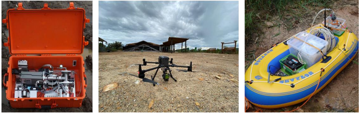
Figure 3. Examples of the Instruments to be used on the field campaigns (Portable Field Spectrometer for Gases, Drone for DEM and Land Use Assessment, Radon Equipment built on a boat).
